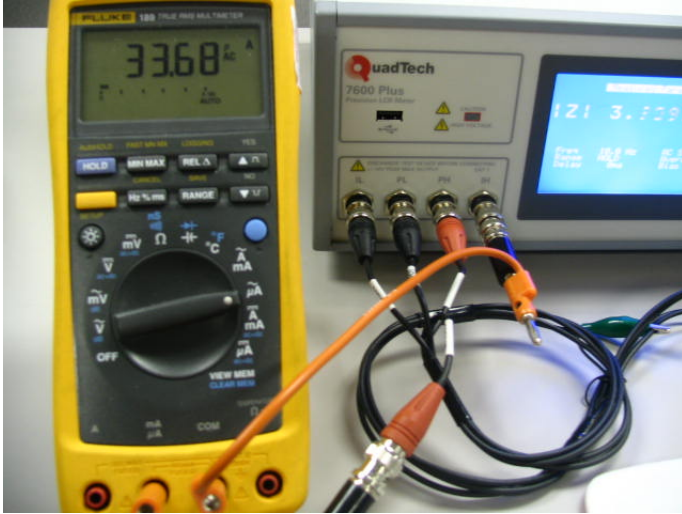
Current Measurement using Fluke 189 Multimeter
