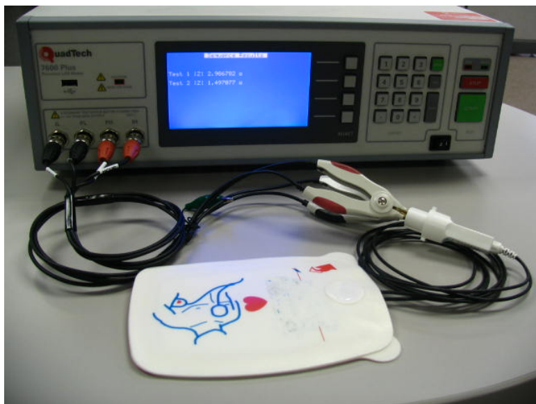
7600 Plus Connected to DF Pads
